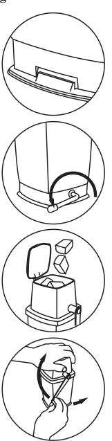
Ensure that the suction cup base is clipped securely to the ice container.
