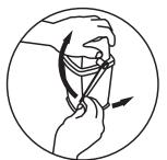
While holding the lid closed on top of the Ice Crusher, turn the handle to crush ice. Turn counterclockwise for coarse ice or clockwise for finely crushed ice.
