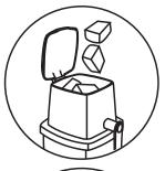
Fill the hopper with ice cubes and close the hopper.
