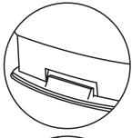
Ensure that the suction cup base is clipped securely to the ice container.
