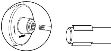
Strainer notches should line up with motor drive shaft keys.
