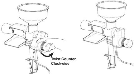
5. You will know the motor is correctly in place when the motor latch is secure around the strainer body (see diagram below) and the drive shaft
